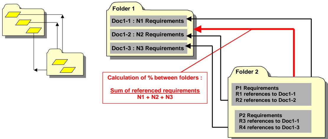
In the case of coverage links between a high level document and a lower level folder, the high level document behaves like if it has combined coverage links with the documents in the lower level folder. When a high level document, or an element (section, requirement, etc.) of the high level document is selected, Rhapsody Gateway displays
