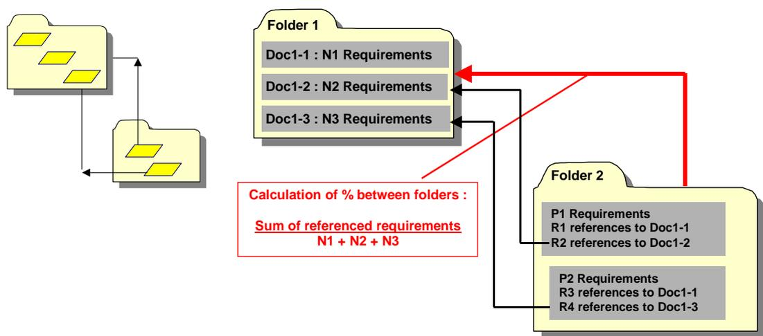
In the case of coverage links between a low level document and a high level folder, the low level document is considered as covering all the documents contained in the high level folder. When a high level document, or an element (section, requirement, etc.) of the high level document is selected, Rhapsody Gateway displays
