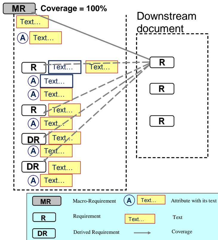
If a macro-requirement references a higher level requirement, all the requirements contained in the macro-requirement are considered as covering the higher level requirement as well.
