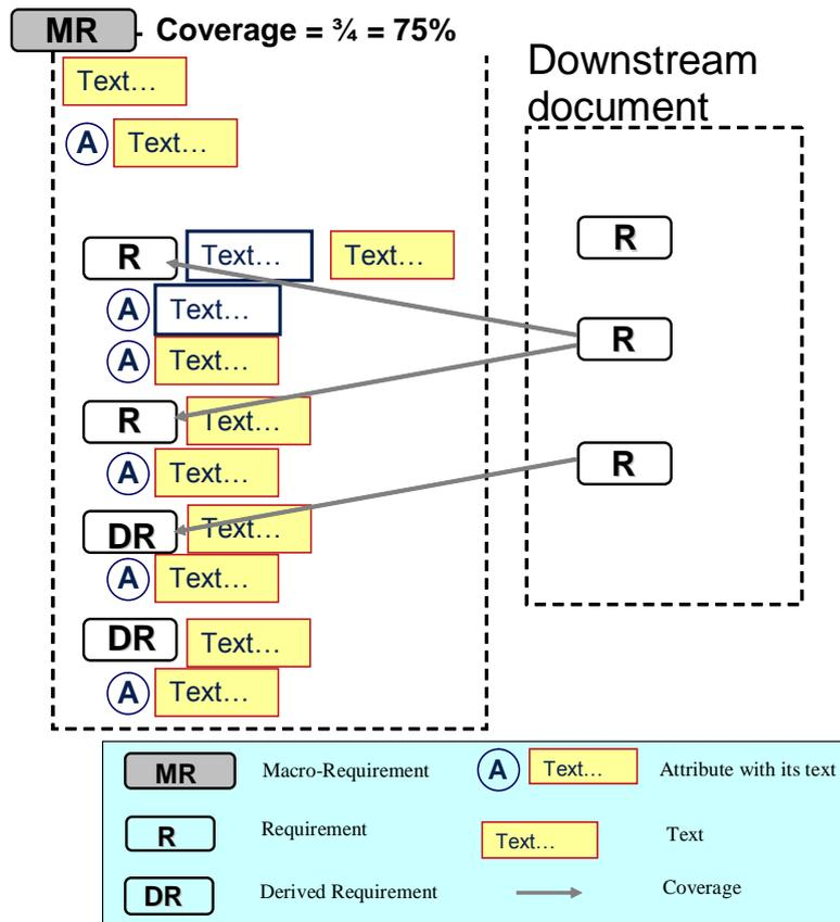
If the macro-requirement is referenced directly by a low level element, it is considered to be 100% covered, and all requirements and derived requirements are considered to be covered by the covering element.
